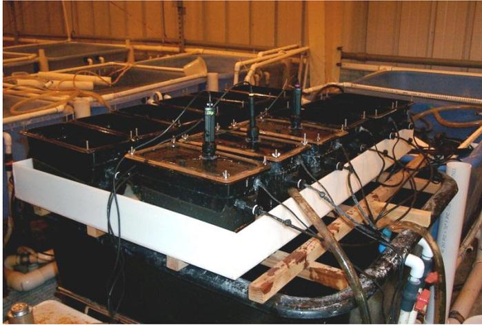
**Figure 45. Static respirometers constructed for this work. The first three units in the foreground with LDO dissolved oxygen probes inserted.**
